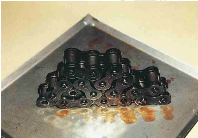
Fig. 1: Roller chain after operation Lubrication with TURMOFLUID® 40 BK
