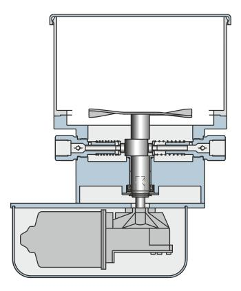
**EasyMatic** is a compact and versatile solution for multiple point lubrication. With the options of various size reservoirs, distributor blocks, pumps and programming capabilities. **EasyMatic** can be configured to suit any specific customer application. **EasyMatic** can pump either oil or grease up to NLGI class 3 and may be used in almost every type of environment thanks to its robust housing.
