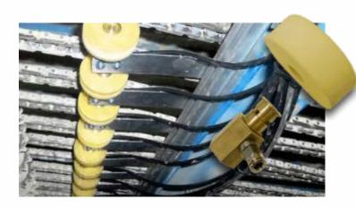
In comparison to manual lubrication, **LUBCON LubeChainSystem** is a cost effective and easy solution for smooth oil application. During operation, the spring-loaded lubricator roll runs on top of the chain. It supplies an optimum oil quantity to chain links without contaminating the production environment.
